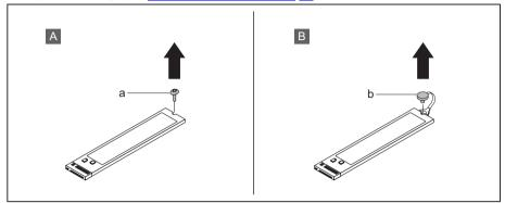
► Variant A with screw: Undo the screw (a).
