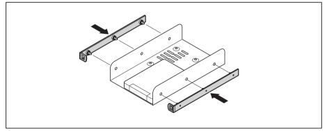
Secure the EasyChange rails to the side of the adapter by inserting the upper pins of the EasyChange rail into the corresponding holes of the adapter.
