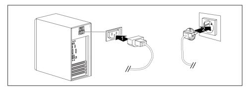
Depending on your device configuration level, plug the monitor power cable into either the monitor socket of the device (1) or a grounded power outlet (2). i
