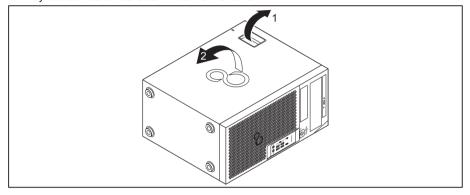
▶ Pull the locking device (1) and swivel the side part in the direction of the arrow (2).
