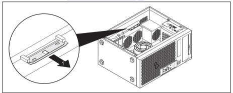
Remove the drive cover from the bracket in the direction of the arrow (1).
