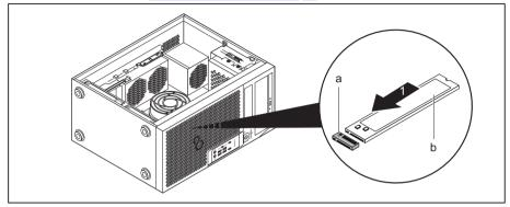
Insert the M.2 module (b) at a slight angle in the direction of the arrow (1) into the slot (a) on the mainboard.
